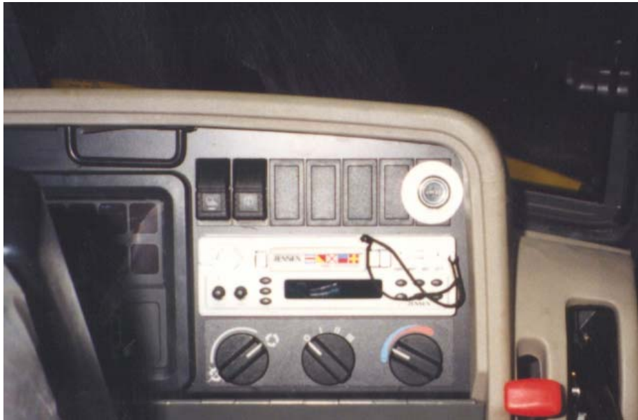
Thermostat location on dash panel.
