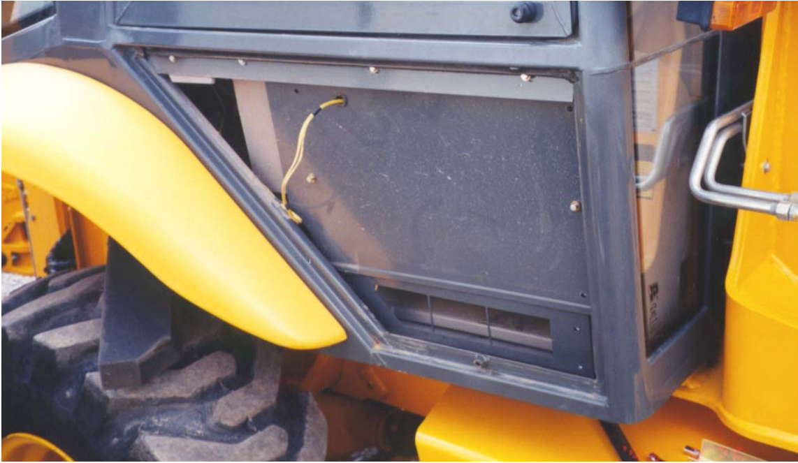
Inner access panel to heater assembly.
