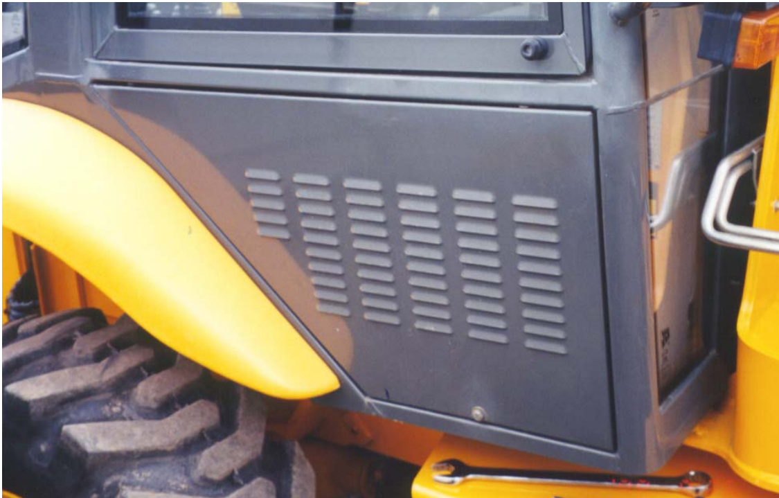
Outer access panel to heater compartment.
