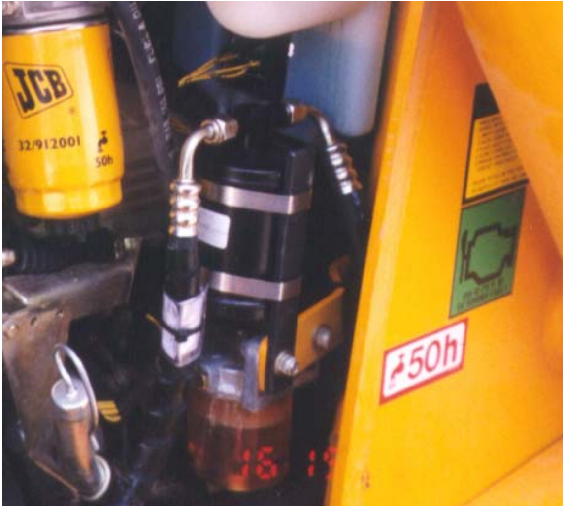
Drier in place on bracket above fuel bowl. Nut showing is for mounting bracket.
